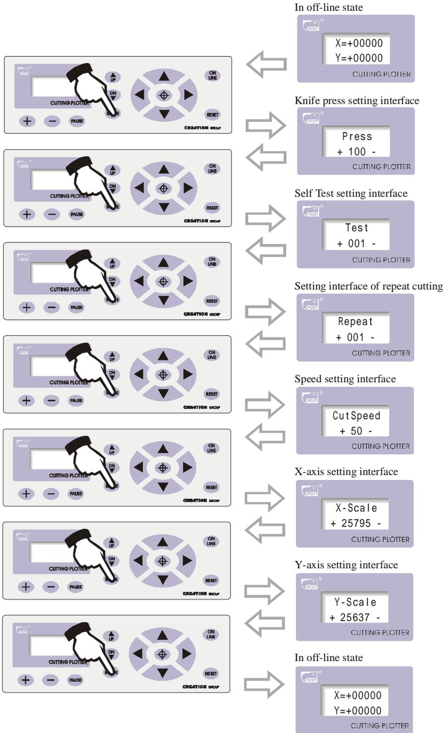
Press “+” and “-” to change the parameters of system. To save present set system parameters, press “PAUSE” button to escape setting mode in off-line state, then press “ON LINE” button once. When switching on machine next time, it will automatically call in the parameters which were set last time as default for starting up.
