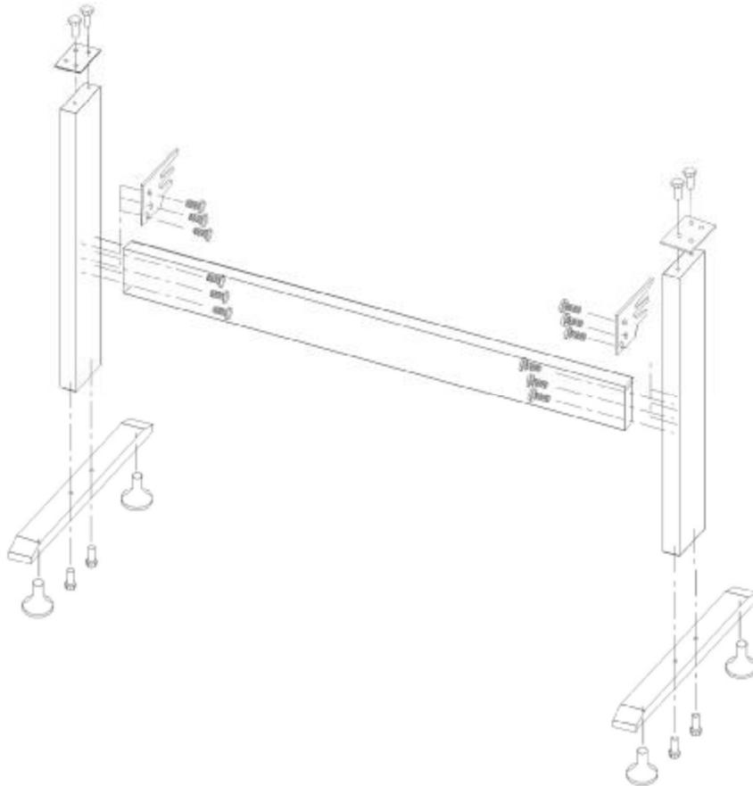
Take parts of the foot stool out of the pack, open the parts bag, install the foot stool as the map shows. After installation place the host on the support with screw hole targeted, then fasten it with screw.
