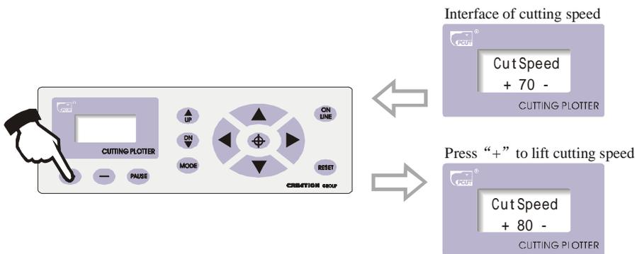
Ø When cutting at high speed, curve may look zigzag, but it is not a trouble, lowering the speed will eliminate the indentation.
